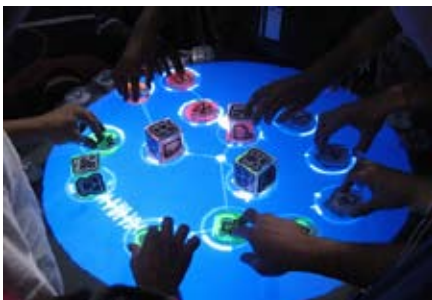
Reactable - Interactive Table to create music using reactivision and fiducials.
